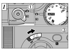
① Set the Mode switch to "\(\mathbf{O}\)" ② and set the Mode dial to "\(\mathbf{AUTO}\)". ③ Then slide the focus mode selector switch to "AF".
